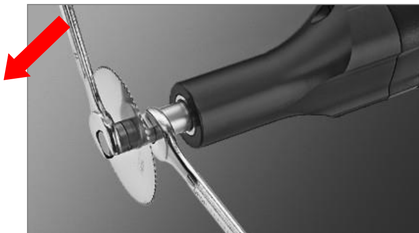
fig. 3 Releasing the retaining screw
