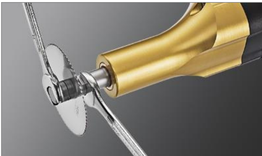
Fig. 1: Releasing the retaining screw
